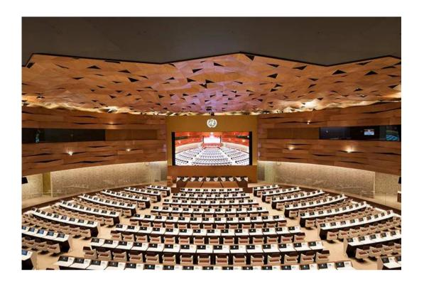
'an important feature of the space is its high-performance acoustics: the parametric modeling software allowed us to simulate the behavior of the surface and its deformation until achieving the volumes dictated by the technical/acoustic requirements of the space,' explains WOOD-SKIN. 'the complex geometries generate an irregular surface that promotes sound diffusion, thereby reducing echo.'
